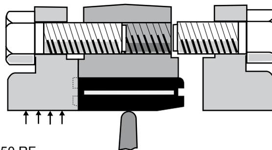
Installation between DIN PN10 and PN16 flanges and ANSI 150 RF
