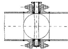
If the stem must be installed parallel to the ground to accommodate dense flowing materials, lower part of the disc should open in the same direction of the flow.
