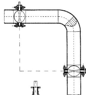
Surrounding space must be provided between the flanges to insert the valve. The disc must be at 95% closed position prior to installing the valve.
