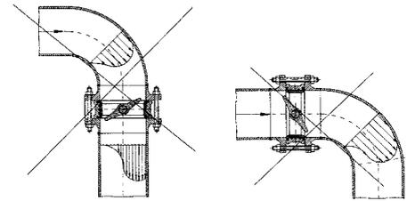
Welded neck type flanges are advised. Otherwise the valves must be centred between the flanges.
