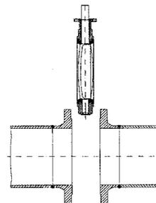
Using scrap pipes is not recommended. The pipes must not be welded to each other at short intervals. The lines connected to the two sides of the valve must be on the same axis to prevent leakage.
