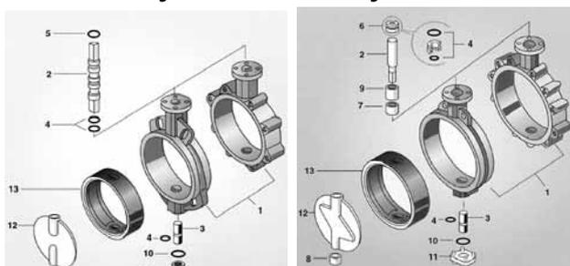
First fully open the valve. Remove the lever system or operating mechanism fitted on the valve. Then screw out plug (11) remove the seal (10). Lift out the top stem (12) followed by the lower stem (3). Force the disc (12) out from the seat (13). Then seat together with the stem o-rings (4). Inspect and/or replace the parts where necessary, then reassemble all items in the reverse order to assembly.
